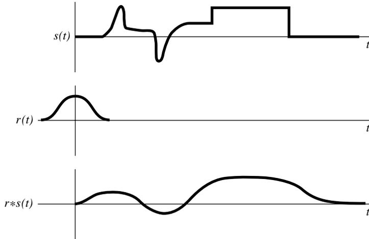
Figure 13.1.1. Example of the convolution of two functions. A signal  $s(t)$  is convolved with a response function  $r(t)$ . Since the response function is broader than some features in the original signal, these are “washed out” in the convolution. In the absence of any additional noise, the process can be reversed by deconvolution.
